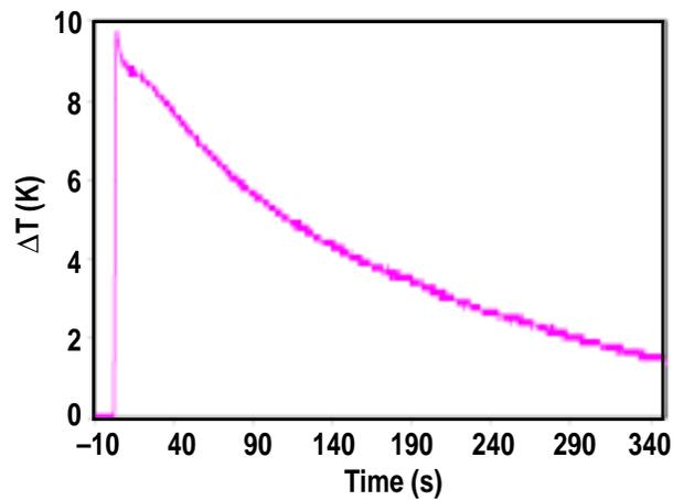
Fig. 2. Typical  $\Delta t$  response for one of the RTDs on the in-line power monitor for a 1 s pulse at a power level of 550 kW.
