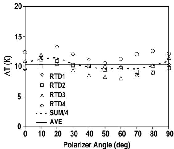
Fig. 3. Rise in temperature measured on the four RTDs mounted on the outside of the in-line power monitor, for 1 s pulses at 550 kW as the polarization is rotated over 90 deg. Also shown is the average for each polarization, SUM/4, and the average of all 40 measurements, AVE.
