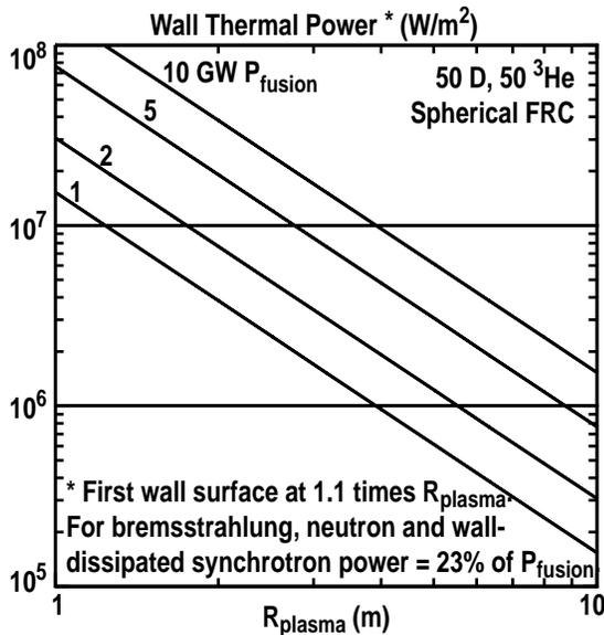
Fig. 2.  $P_w$  vs  $R_p$  with  $P_f$  as a parameter, for  $R_w = 1.1 R_p$  and  $f_{heat} = 0.23$ .
