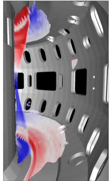
**Figure 1: Coherence Imaging measurement of the line-integrated velocity of carbon ion winds in the boundary of a high performance DIII-D plasma. Velocity data is mostly near the center of the machine where the ion light is brightest. Red denotes positive velocity (into the page) whereas blue is negative velocity. Image courtesy of LLNL.**
