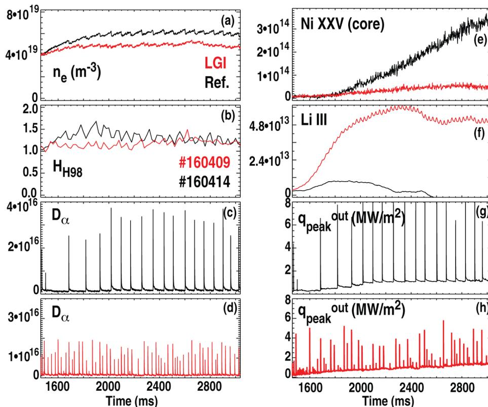
The overall energy confinement tended to decrease with increasing ELM frequency; in some cases, however, the energy confinement could be maintained, e.g. panel (b) using 0.5 mm Li granules.
