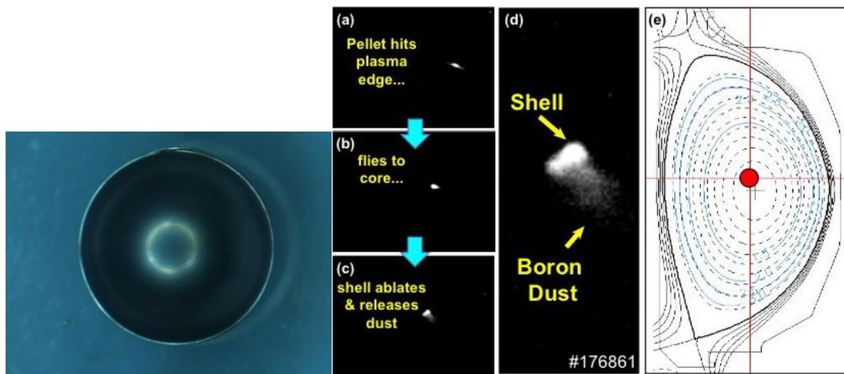
Left: X-ray image of 3.6mm-diameter,  $40\mu\text{m}$ -thick, 30mg B-filled diamond shell. Right: Visible imaging of (a) shell pellet hitting low-field-side boundary of plasma, (b) continuing through plasma toward core, (c) ablating and releasing boron dust in core. (d) Expanded view of (c), highlighting shell and dust. (e) Plasma cross-section with red dot indicating pellet location at time of dust release in (c). Injection velocity  $\approx 230$  m/s. *Image courtesy of ...*
