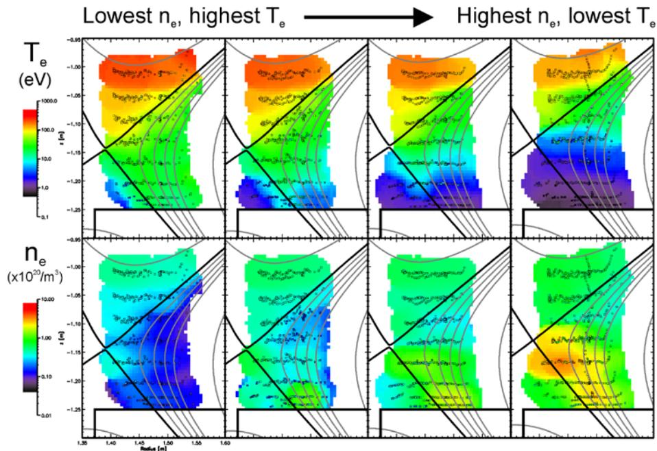
Figure 1: 2-D electron temperature (top row), and density (bottom row) for each of four plasma boundary densities increasing from left to right as measured by divertor Thomson scattering in DIII-D. Small squares indicate measurement locations mapped to the displayed magnetic equilibrium.
