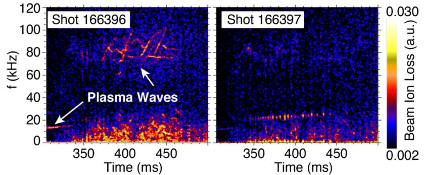
**TURNING OFF TROUBLESOME WAVES:** Spectrograms of measured beam ion loss. Both plasma shots feature the same total beam power, but the shot shown on the right utilizes a beam voltage program that greatly reduces the amplitude of coherent plasma waves. Adapted from [D.C. Pace, et al., Nucl. Fusion 57, 014001 \(2017\)](#).
