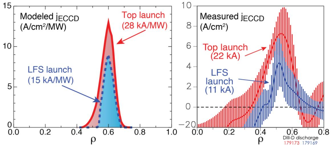
Figure 2: The prediction of doubling the off-axis current-drive efficiency due to more selective wave energy damping via a top-launch ECCD system has been validated by recent experiments at DIII-D. Left is prediction using the CQL3D quasi-linear Fokker-Planck code and right are measurements. Credit: Xi Chen, DIII-D National Fusion Facility
