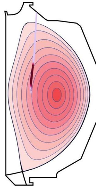
*Figure 1: The red line shows the driven current density along the microwave trajectory in a DIII-D plasma, with the darker red showing where the larger current is driven into the plasma. This figure was modeled with the TORAY-GA ray-tracing code. Credit: Xi Chen, DIII-D National Fusion Facility.*
